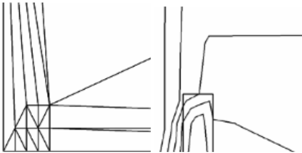
Fig. 3. The initial mesh and the magnetic flux lines for the one coil model.
